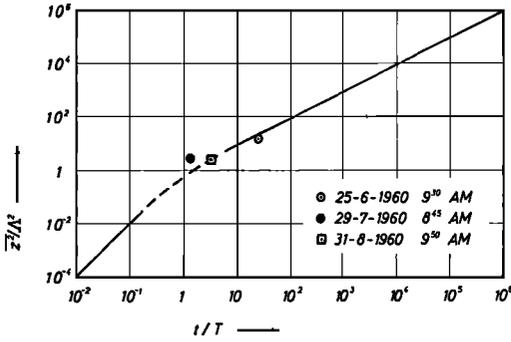
Fig. 1. Example of the universal diffusion pattern in homogeneous, isotropic, fully developed, and stationary turbulence.
