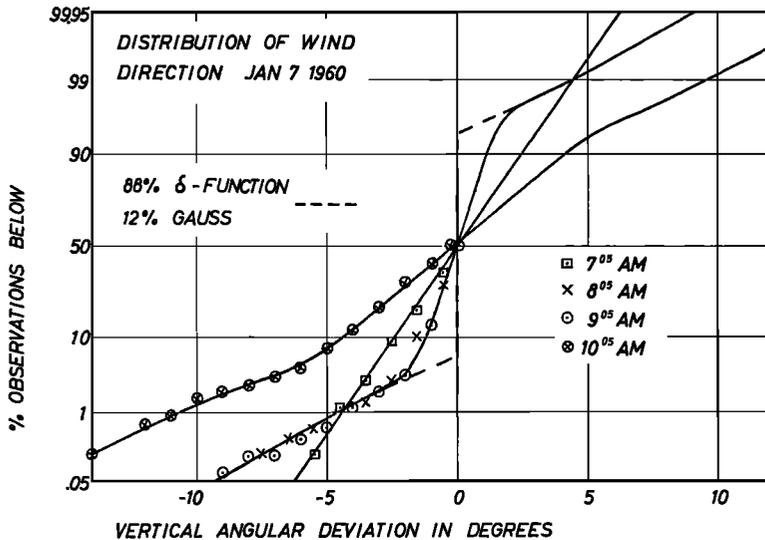
Fig. 2. Probability that the vertical angular deviation from the mean is smaller than a given value plotted against the deviation on graph paper resulting in straight-line plots if the probability distribution is Gaussian.
